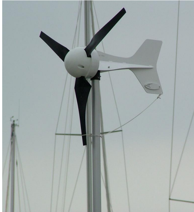
Fig-16: Tethering the rotor blades using the hole on the tail-fin
