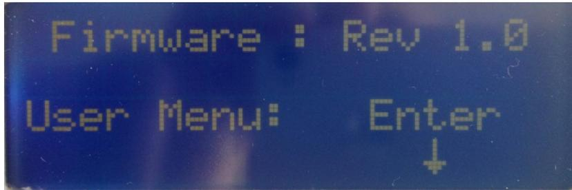
Press ENTER to view the programming menu. Use the UP and DOWN keys to scroll through and ENTER to select an option. A cursor indicates the option available to select.
