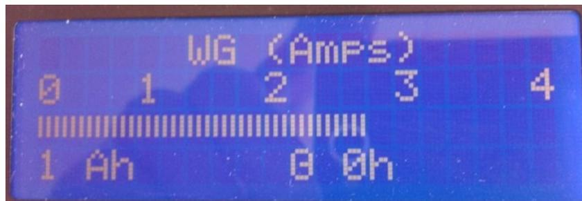
WG or PV or Total is displayed by scrolling through UP and DOWN
