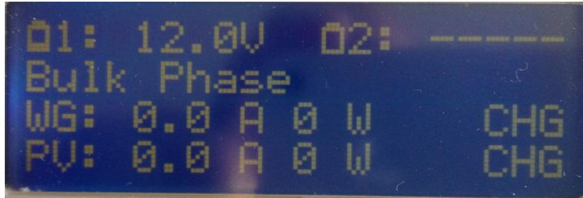
Battery 2 is shown as not connected.
