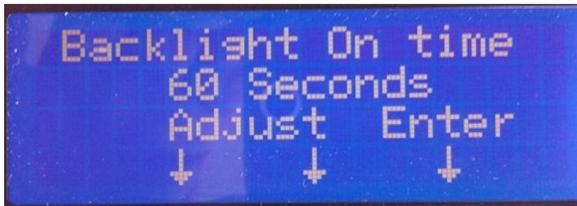
Adjust the seconds using the UP and DOWN buttons to the desired duration, one press adjusts one second. Press ENTER to save this time to non volatile memory and return to the programming menu.
