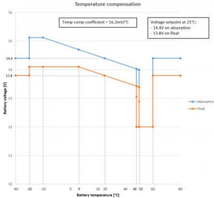
With a temperature sensor installed to the User I/O connection block; the actual battery temperature will be used for compensation; throughout the day.
