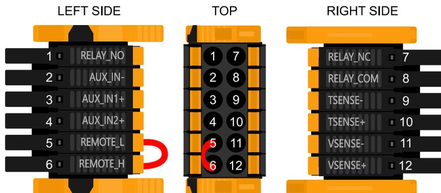
User I/O Connector is located on bottom left side of connection area, diagram shows 3 perspectives. Left Side - Top - Right Side
