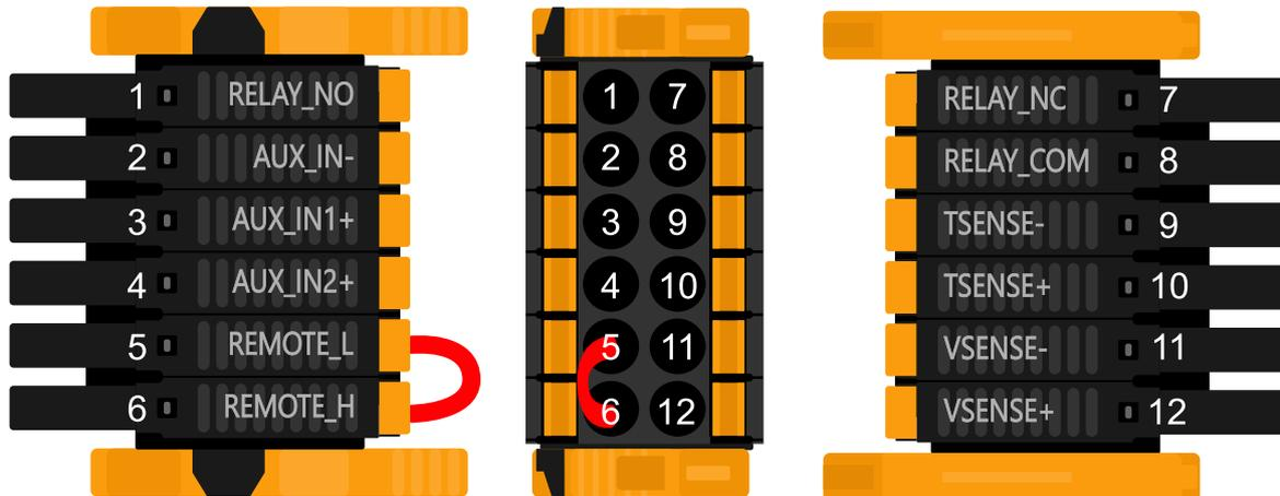
User I/O Connector is located on bottom left side of connection area, diagram shows 3 perspectives. Left Side - Top - Right Side
