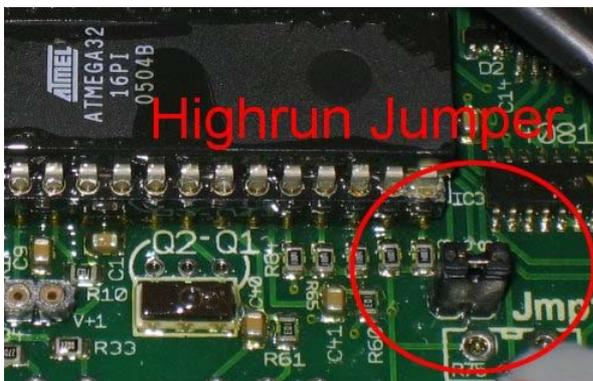
In order to set the Battery High Run function set the jumper as shown in above picture. This will increase the Low Voltage Disconnect settings to 12,3 / 24,6V and the re-start voltages to 13,3 / 24,6V to allow pumping only when the batteries receives charging current from the solar array. The lifetime of the battery will be increased considerably as cycling is avoided.
